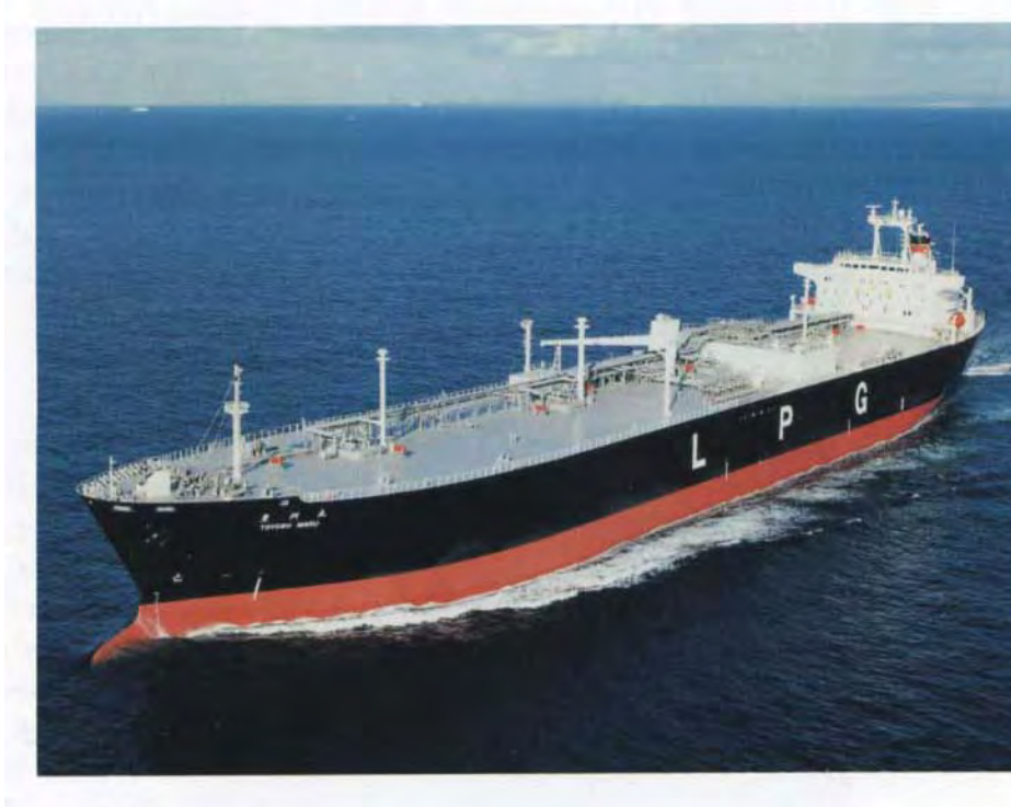
Figure 4.6: A LPG tanker – CO 2 could be transported in a similar way. Courtesy of Mitsubishi Heavy Industries.
