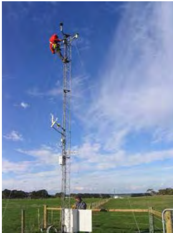
Figure 9.12: CO 2 flux station (courtesy of CO2CRC).
