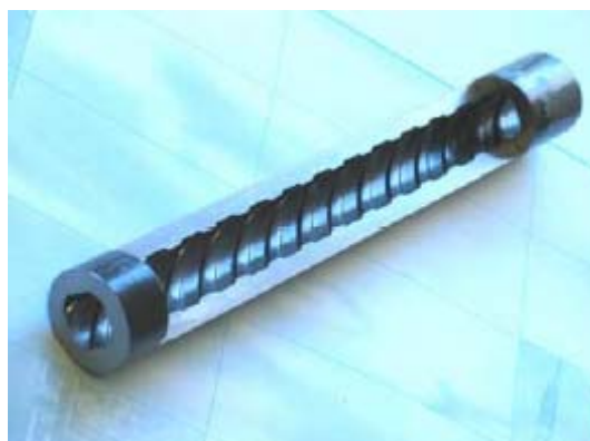
Figure 14 Sample of a Boiler Tube with Rifled Inner Wall
