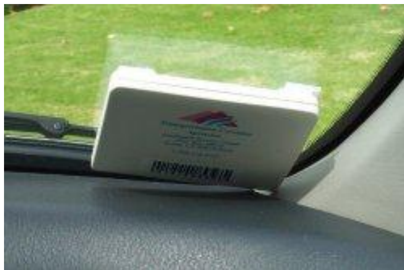
Fig. 1.2.4.1.2. RFID-tag for vehicle identification
