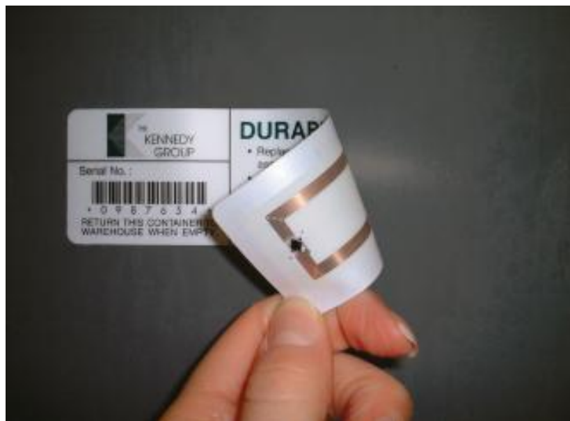
Fig. 1.2.4.1.3. Combination of a RFID tag and a bar code
