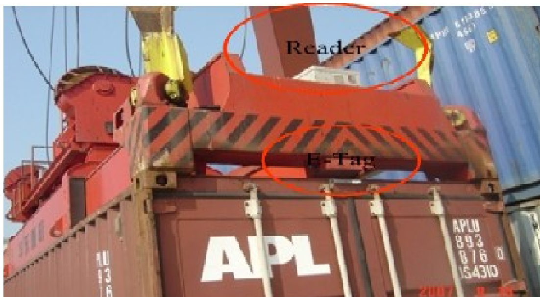
Figure 6 Reader installed on the gantry crane and the E-tag on the container
