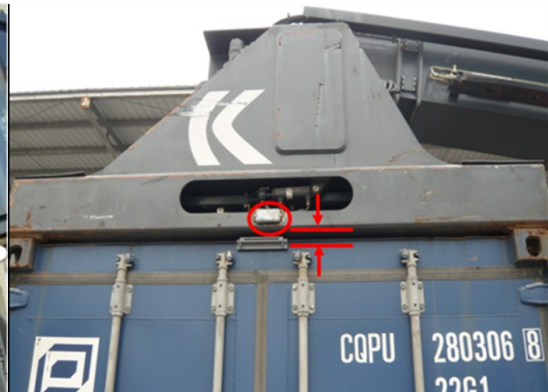
Figure 6 Reader fixed on moving machines
