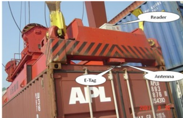
Figure 5 Reader and antenna fixed on gantry crane
