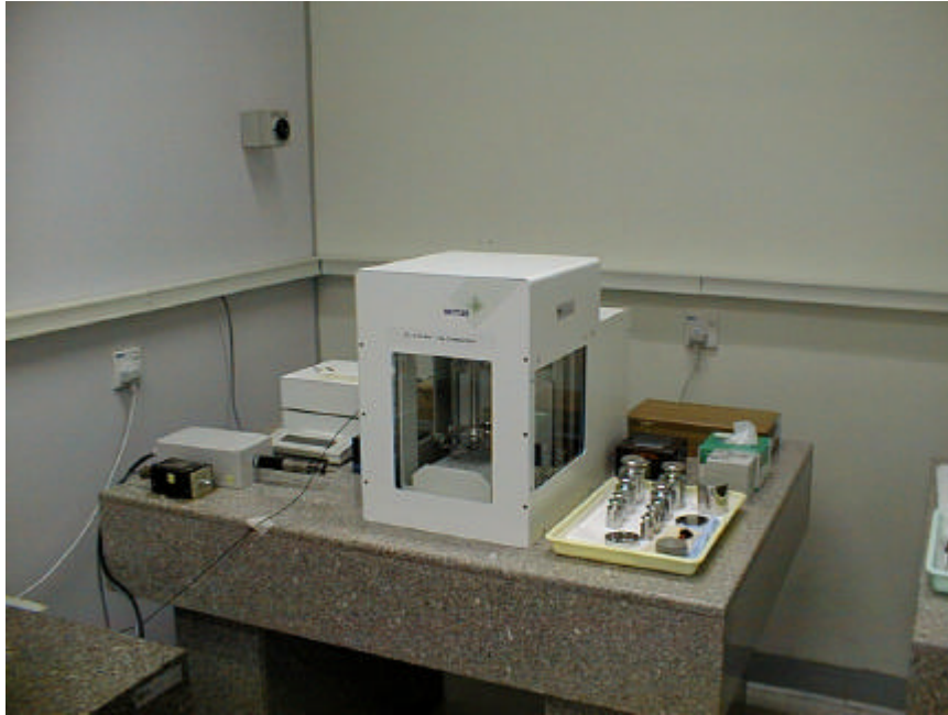
Figure 5 : A 1 kg Mass Comparator used in the mass comparisons from 200g to 1 kg.
