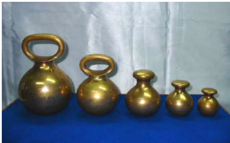
Figure 2 : ‘Imperial’ pound standards issued to inspectors of weights and measures in the 1960s ( L to R : 14, 7, 4, 2, 1 lb)
