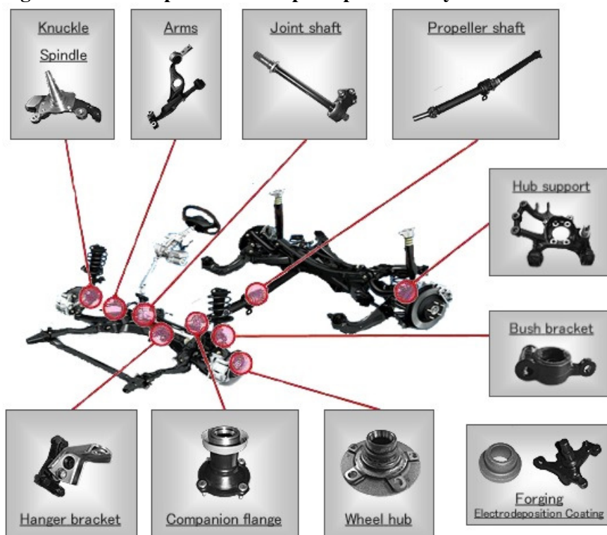
Figure 14.2. Examples of chassis parts produced by firm A
