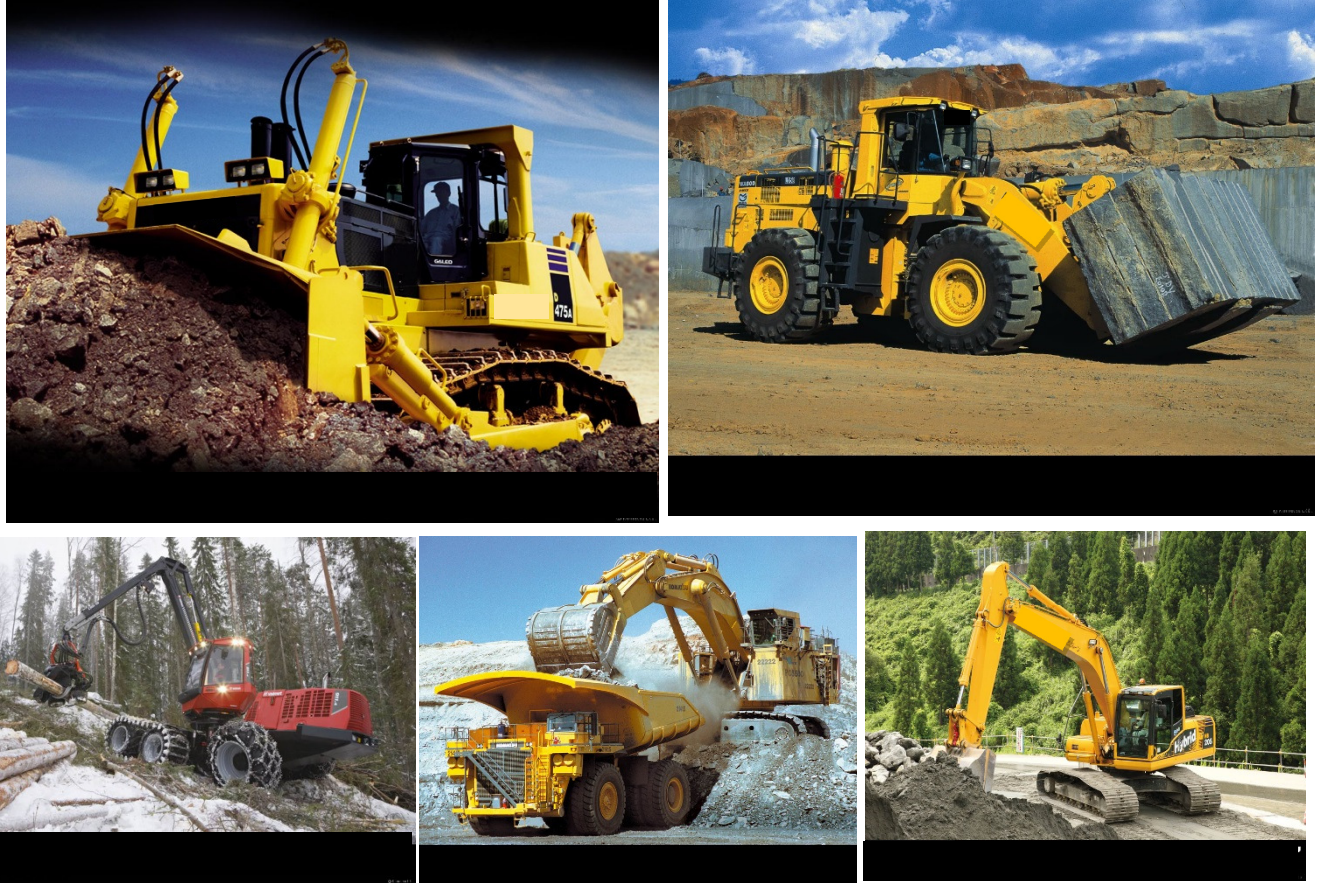
(Upper left: Bulldozer; Upper right: Wheel Loader; Lower left: Harvester; Lower middle: Mining Equipment; Lower right: Hybrid excavator) Source: Courtesy of the firm
