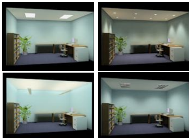
Figure 4 | Lighting distributions from different luminaire types
