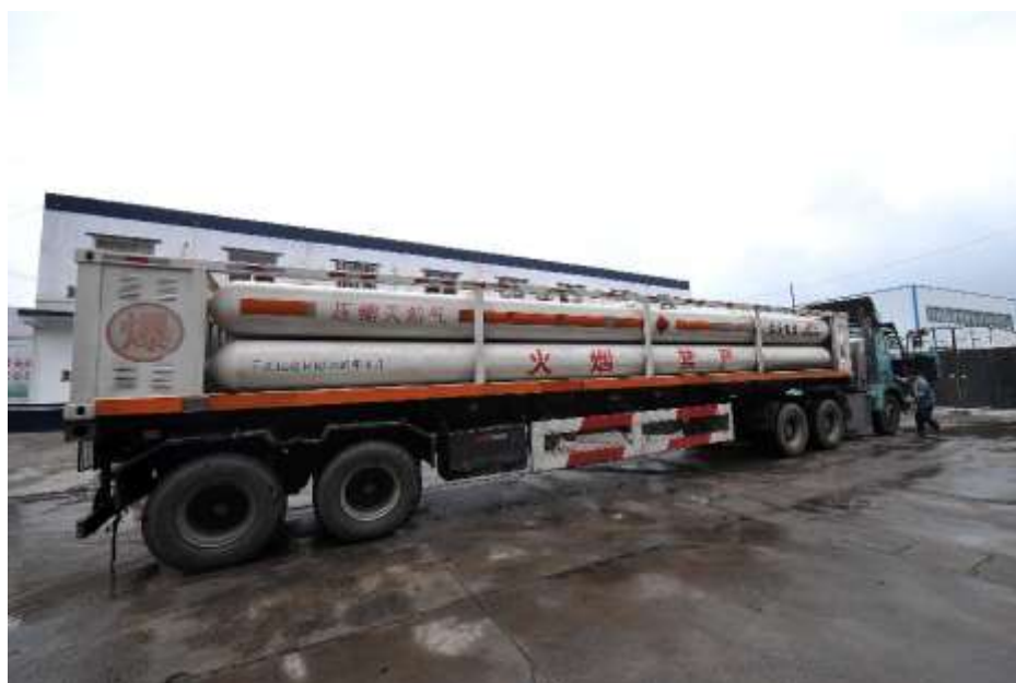
Fig.2-14 CNG tank car in Jincheng
