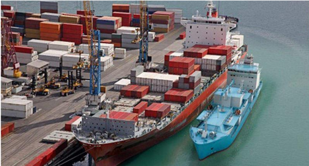
Figure 24: LNG Bunkering Ship Filling Container Vessel 47
