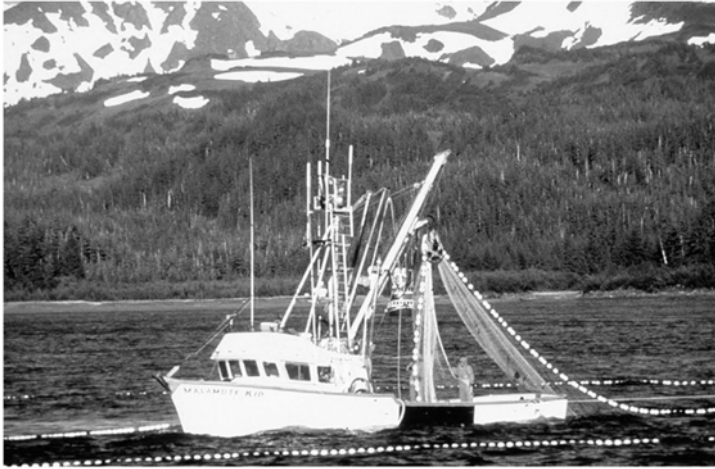
Figure 11.04 Fishing vessel pulling in a purse seine net. The floats, net, and circular enclosure are all visible (courtesy of NOAA).
