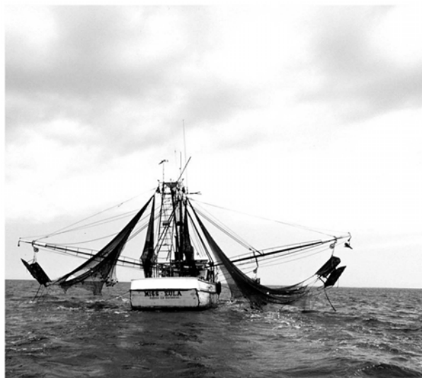
Figure 11.03 A shrimp boat rigged with otter trawl gear. Floats, nets, and doors are all visible (courtesy of NOAA).
