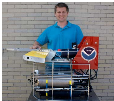
Figure 6. The Mariner Shuttle Mk II, Instrumentation: CTD; Plankton Sampler; Fast Repetition Rate Fluorometer with a PAR sensor to study photosynthesis and primary productivity; fluorometer to measure both chlorophyll and turbidity; nitrate sensor dissolved oxygen sensor. The system is towed at up to 8 kts and can adjust the flight pattern match the bottom depth.
