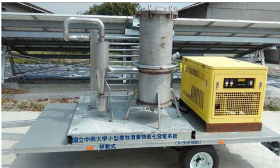
Fig. 4.4 10 kWe small-scale mobile downdraft biomass gasification-based power system
