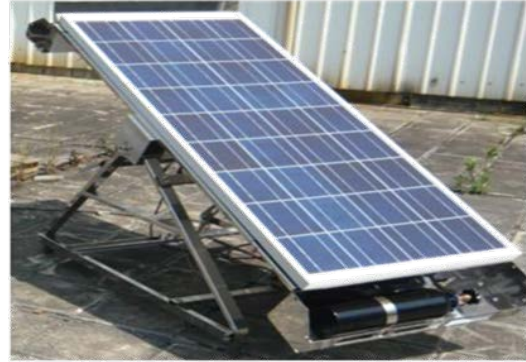
Fig. 4.3 Automation tracked solar energy system
