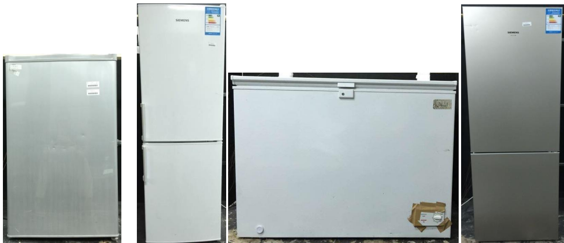
Figure 2-1 Test sample of upright refrigerator, Upright refrigerator-freezer, Chest freezer, Upright frost-free refrigerator-freezer (from left to right)
