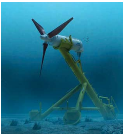
Figure 17. Andritz Hydro – Hammerfest (Germany – Norway) HS1000 tidal turbine 1MW at 2.7m/s, deployed at the EMEC
