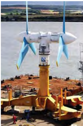
Figure 21. Atlantis Resources Corporation (UK) AR1000 1.0MW at 2.65 m/s tidal turbine, deployed at the EMEC
