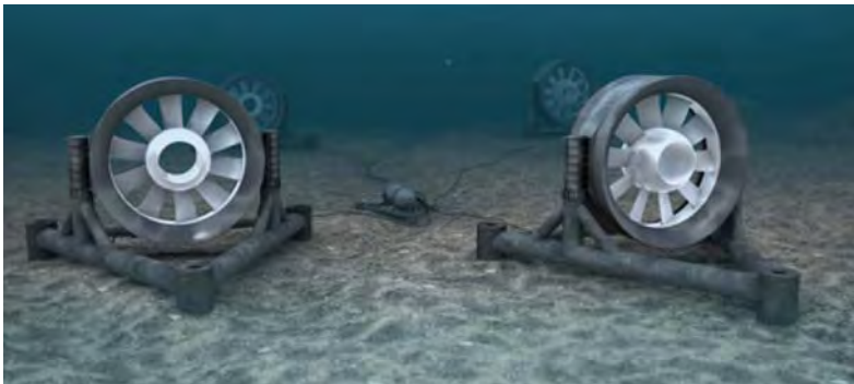
Figure 23. Open Hydro / EDF project: a single 16m turbine rated at 2MW followed by an array of grid-connected units, deployed at Paimpol-Brèhat tidal farm in Brittany, France
