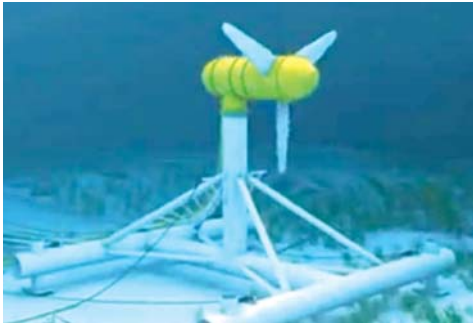
Figure 20. Voith Hydro (Germany) 1.0MW at 2.8m/s tidal turbine, deployed at the EMEC, 110kW scale model tested in Korea
