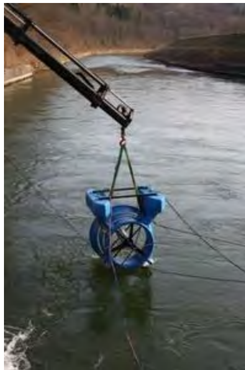
FIGURE 9-24 : Turbine for location with free flow
