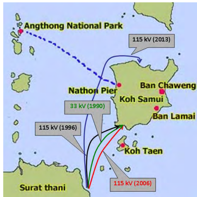
FIGURE 2-2 Existing Submarine Cable for electrical power supply
