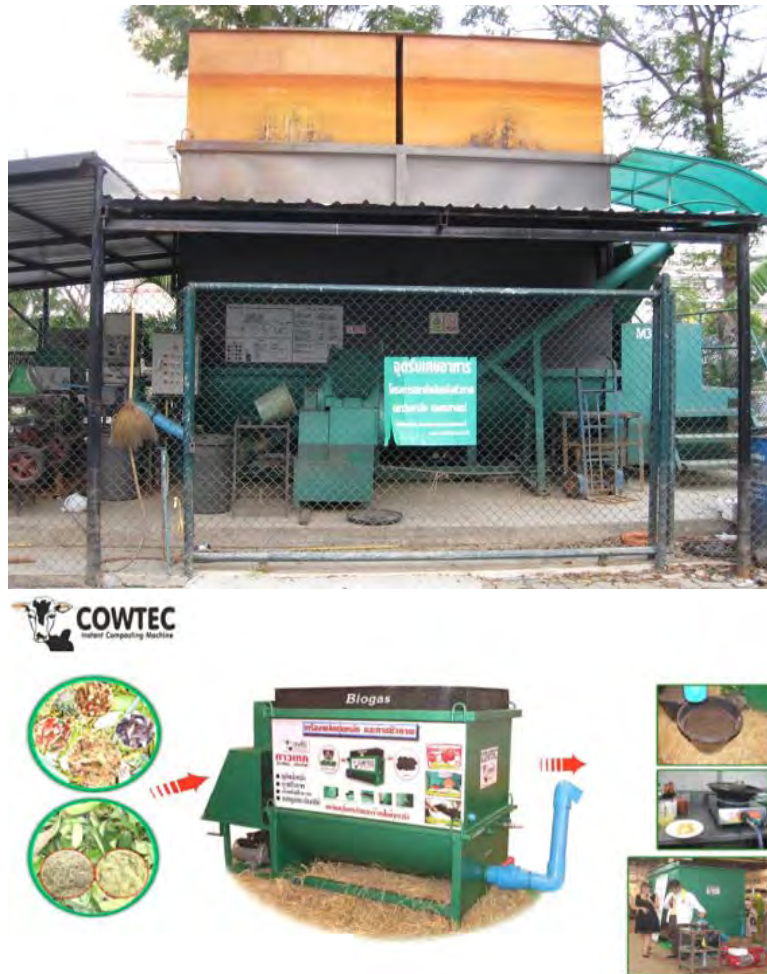
FIGURE 10-9 : Organic fertilizer and bio-gas production center at Kasetsart University and biogas production machine
