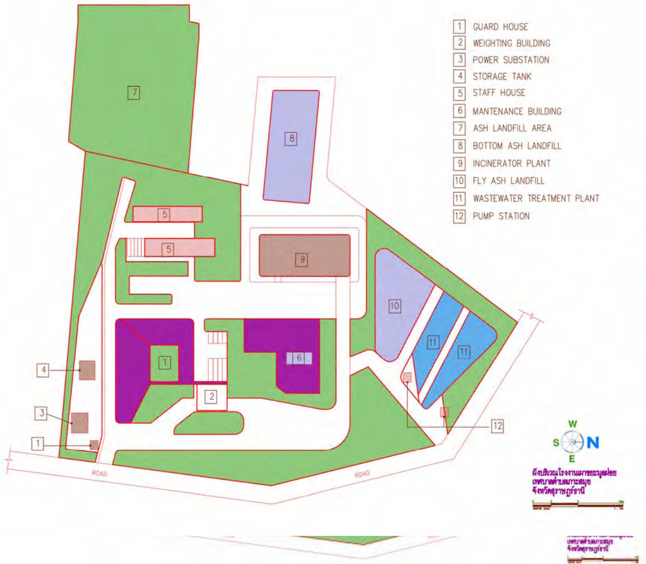
FIGURE 10-5 : Layout of existing incinerator plant
