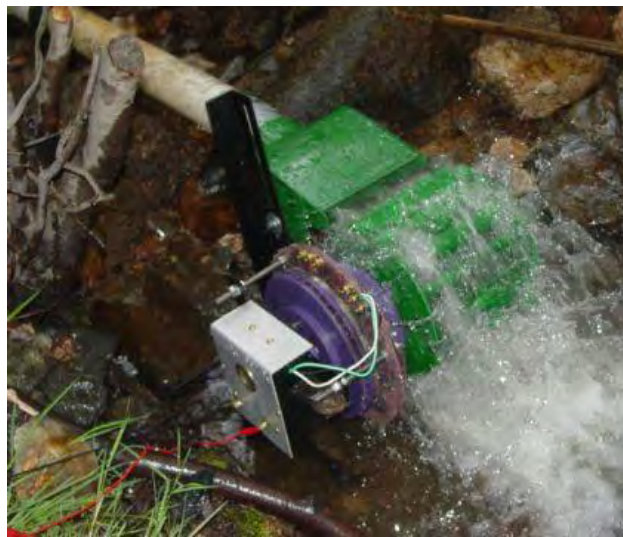
FIGURE 9-21 : Water wheel for micro hydroelectricity power plant
