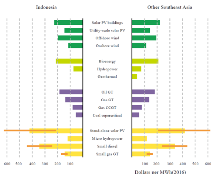
Figure 1-3 Comparative cost of power generation in Indonesia and other Southeast Asian economies
