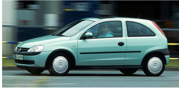
Figure 5. Smooth Wheel Covers Reduce Drag (shown on a GM Opel Corsa Eco) (Photo courtesy of General Motors)
