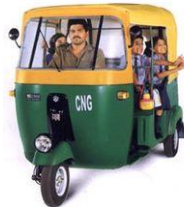
Figure 7. Three-wheel Bajaj rickshaw with a two-stroke engine powered by compressed natural gas. (Photo: www.dinesh.com )
