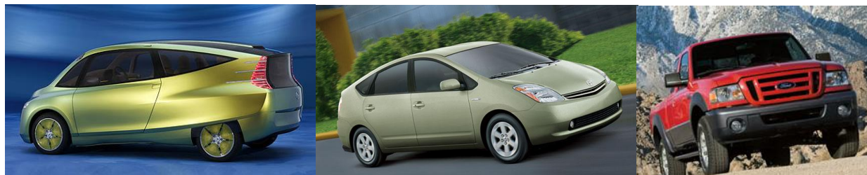
Figure 4. Coefficient of Drag (Cd) on Selected Vehicles. From left to right: Mercedes-Benz concept car (0.19), Toyota Prius (0.29), and Ford Ranger ( \geq 0.4 ). (Photos courtesy of DaimlerChrysler AG, Toyota Motor Corporation, and Ford Motor Company, respectively.)
