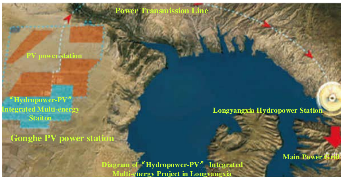
Fig. 3-2.1 Diagram of “Hydropower-PV” Integrated Multi-energy Project in Longyangxia
