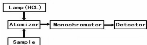
Figure of simple single element nondispersive AFS instrument
