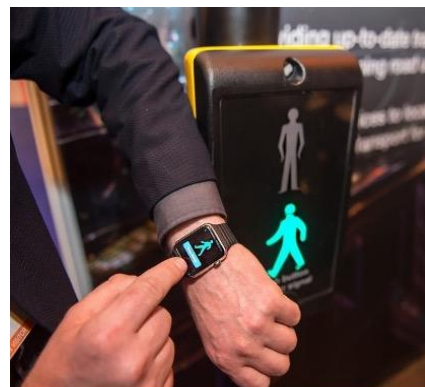
Figure 14: Neatebox connects pedestrians to traffic lights.
