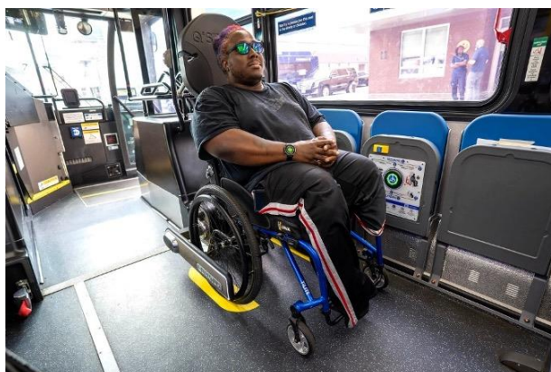
Figure 16: Q'straint Quantum Wheelchair Self-Securement Station
