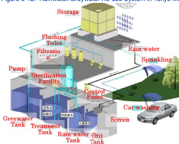
Figure 8-12: Rainwater/Greywater Re-use System in Tokyo Midtown
