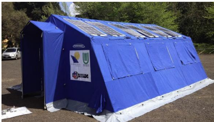
Fig. 3.1 Temporary shelters six crystalline silicon thin-film photovoltaic modules.
