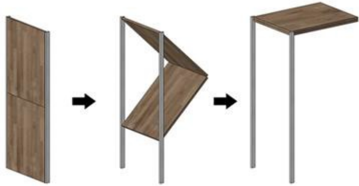
Fig.4.14 Schematic diagram of sliding door opening and closing mode Source: APSEC
