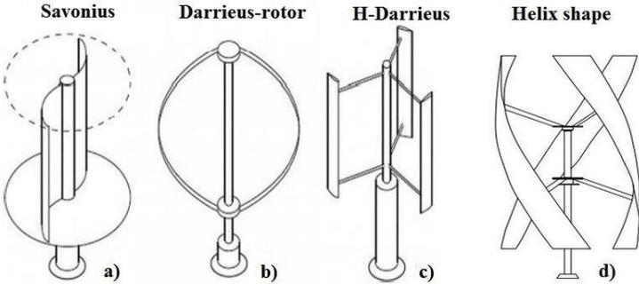
Figure 90: Four of the most common vertical axis wind turbines for urban environments
