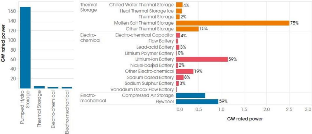
Figure 99: Global operational energy storage power capacity by technology (2017)
