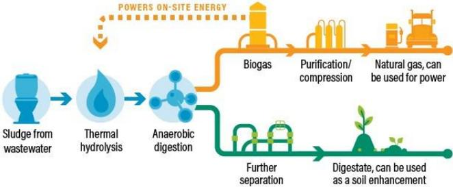
Figure 94: Wastewater-to-energy scheme
