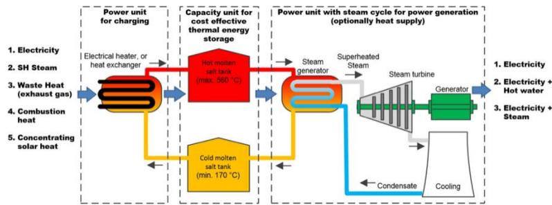
Figure 100: Concentrated Solar Power (CSP) using molten salt as storage medium
