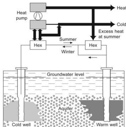
Figure 104: Aquifer thermal energy storage (ATES)
