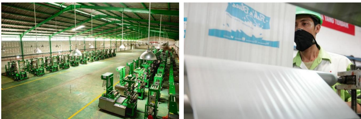
Figure 14. Bioplastic sheet production machine made from bioplastic pellets
