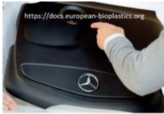
Bio-based polyamide car engine cover
