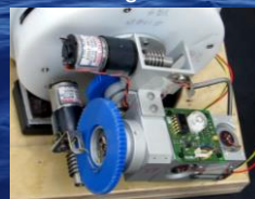
Sensors with in-house leveling device
