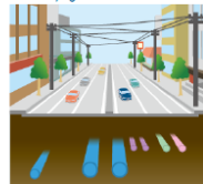
Direct burying and overhead line methods
