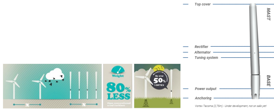
Fig. 4.3-4. Feature of bladeless wind energy system Source: Vortexbladeless.com
