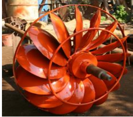
Metal runner for an improved water mill Source: Ashden Awards Website
