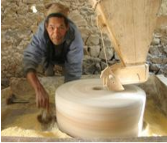
Grinding maize with an improved water mill
