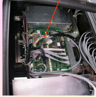
Lead sealing the regulator of oil meter
