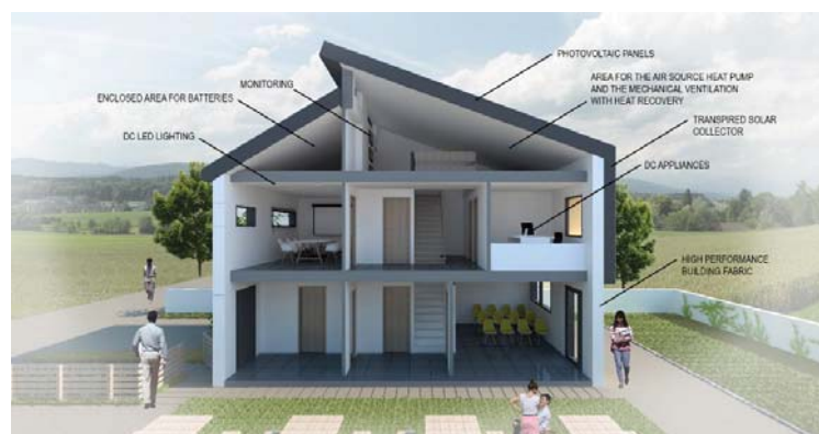
Fig. 3-18 Building energy management system (BEMS)
