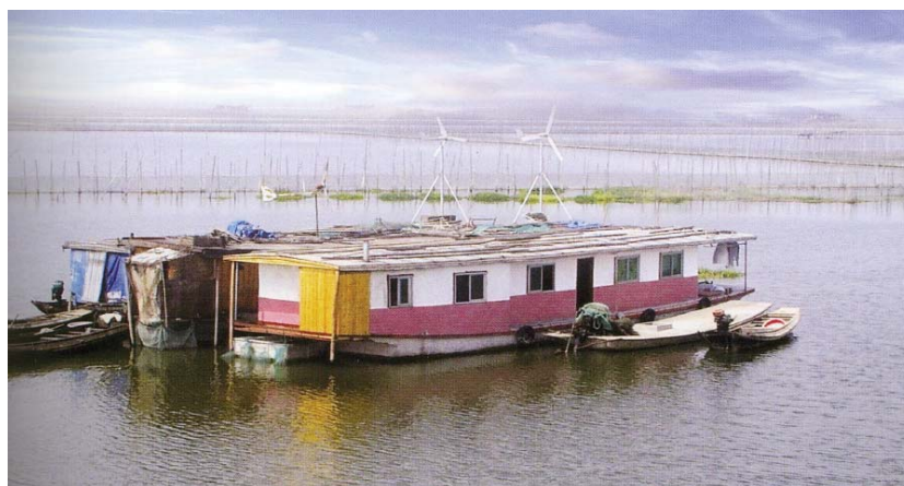
Fig. 2-14 Mini-size wind power system on boat
