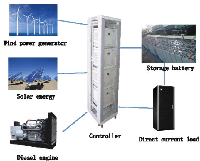
Fig. 2-16 Wind-solar hybrid system
