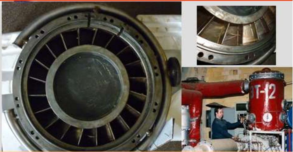
Diaphragm with slots in nozzle blades for steam injection
