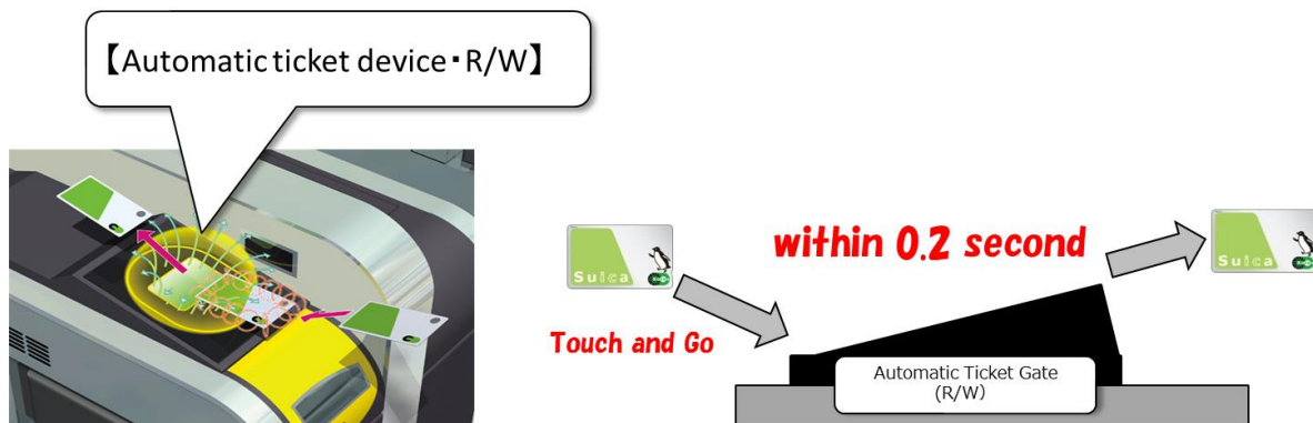
Figure 2-36: High speed processing of IC cards
