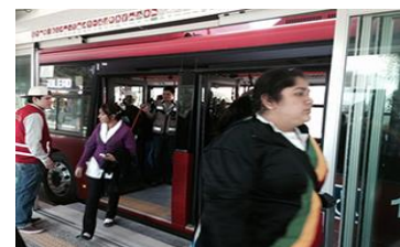
Figure 2-56: Ecovia, low floor bus
