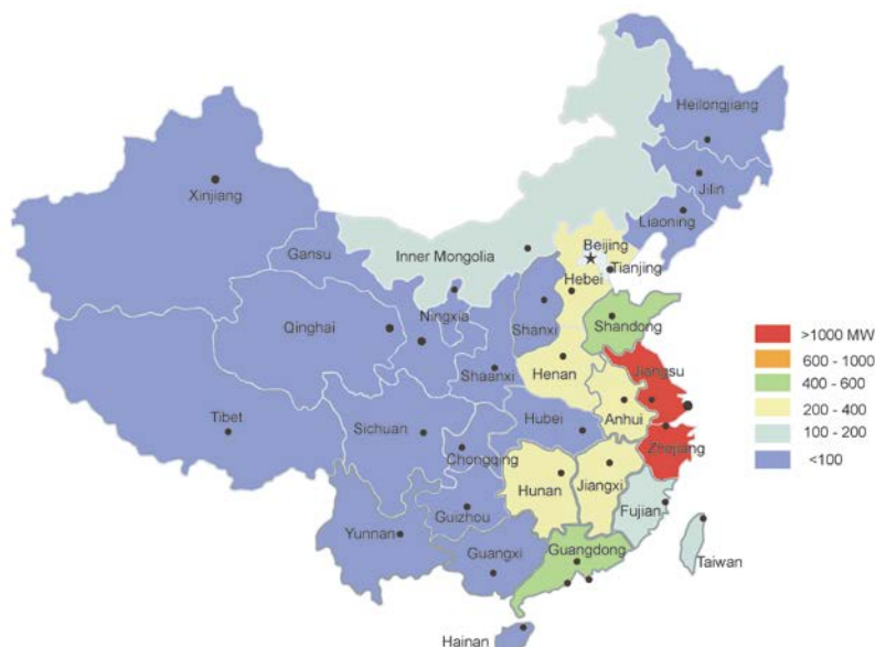
Fig. 3-9 Distribution of cumulative installed capacity of distributed PV by the end of 2015
