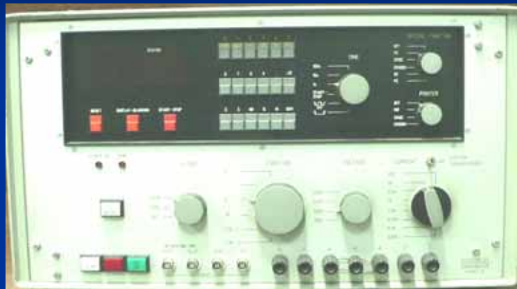
ZERA IML03-3 Class 0.01 single-phase electric energy standard device
