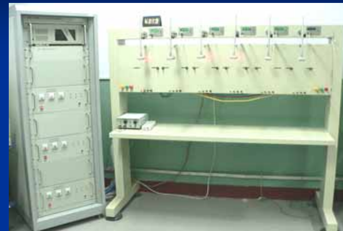
NST-3500 Class 0.03 three-phase electric energy standard device
