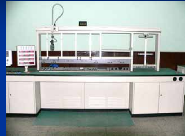
ZERA ED7186 Class 0.03 three-phase electric energy standard device
