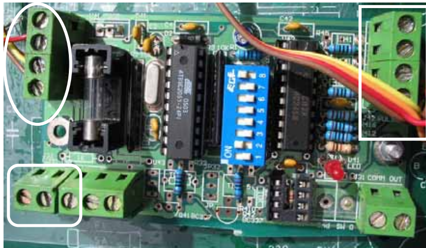
Figure 4. The additional device for manipulate measuring data of fuel dispensers
