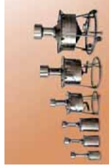
A set of volume standards with capacity from 2L to 200L. Accuracy class: 0.1
