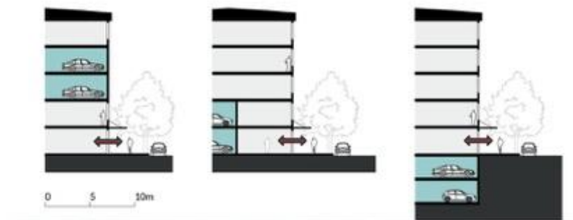
Figure 2.2: Position of car parking on different levels and in different positions allows a more diverse street
