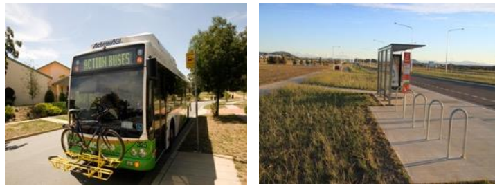
Figure 6.7: Example of the cycle racks on buses in Canberra, Australia, and cycle parking areas for privately
