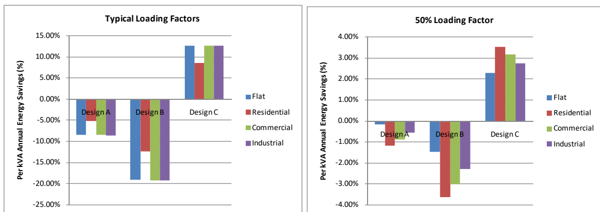
Figure 6-25: Per kVA Annual Energy Savings in % from Adoption of IEC 60076-20 in MEA's Networks
