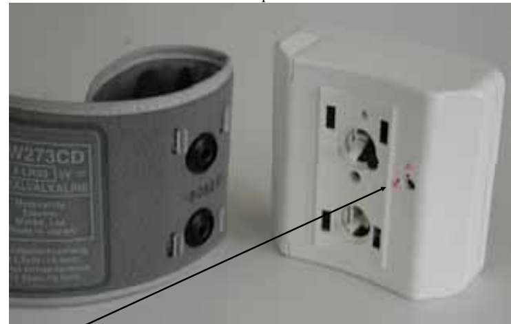
The valve has to be turned in the positon c (close) for verification and after verification back to o (open) for normal use
