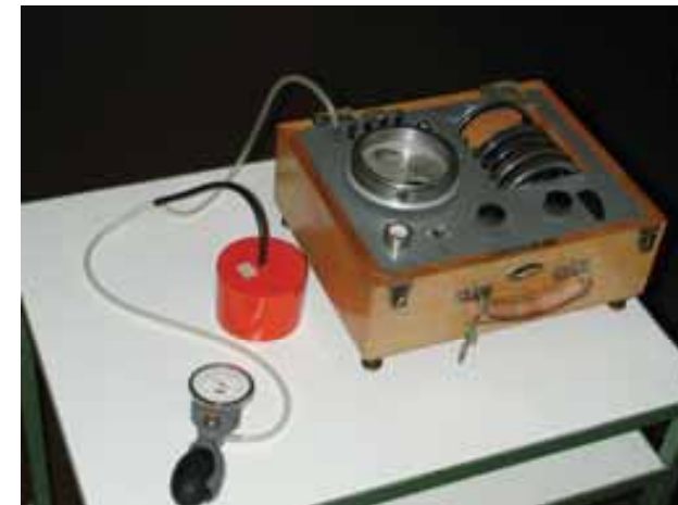
Figure: Measurement setup to determine the limits of error of the cuff pressure indication (aneroid manometer)
