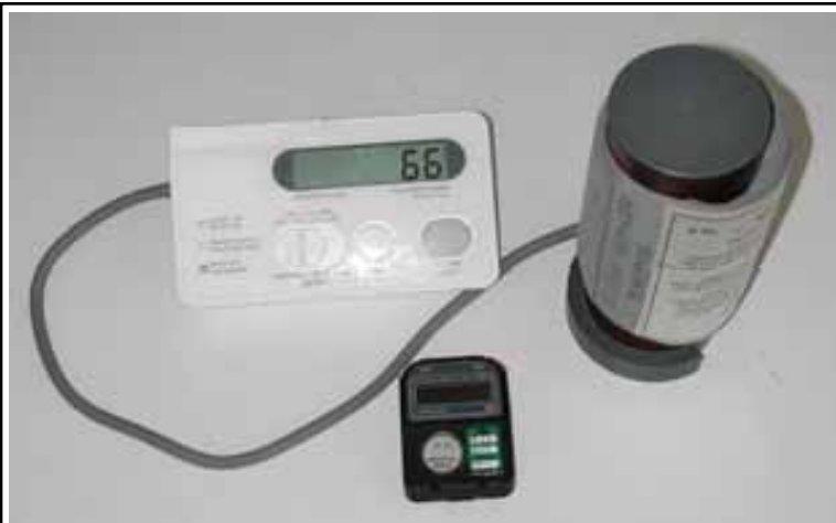
Figure: Air leakage test set-up (a pump has to be included, which is not shown here)
