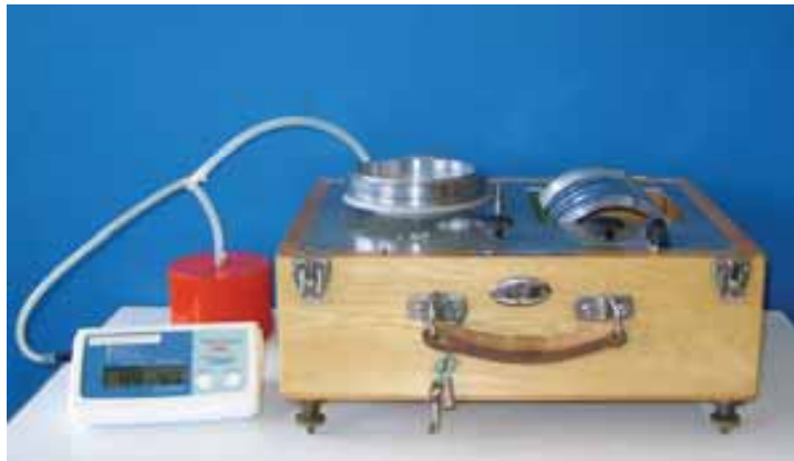
Figure: Measurement setup to determine the limits of error of the cuff pressure indication (home use device)
