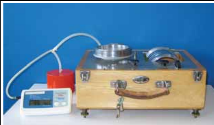
Figure: Measurement setup to determine the limits of error of the cuff pressure indication (home use device, please note: the pressure is displayed in the systolic and diastolic field)
