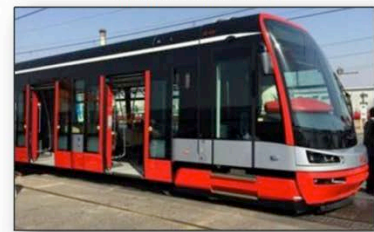
World's first light rail tram, powered by a Ballard fuel cell module
