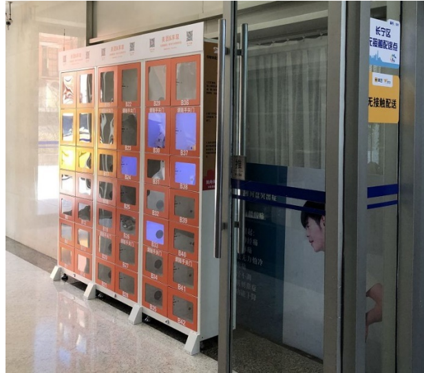
Figure 29. Smart Food Cabin equipped with ultraviolet disinfection and heat preservation functions 68 .
