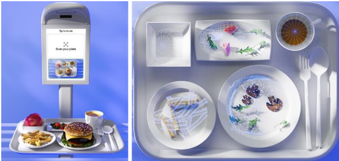
Figure 6. Nuvilab's AI food tray scanner that measures plate waste and personal intake data.
