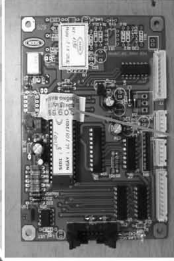
Seal on the program IC
