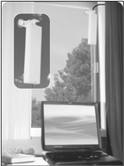
Photo 2-5: Antenna on Residential Window
