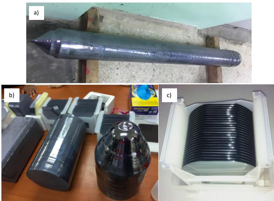
Photo 1 : a) Silicon Ingot, b) Cut part of Silicon Ingot and c) Silicon Wafer
