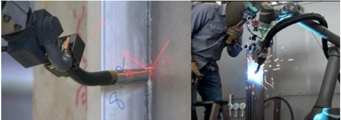
Figure 14. Welding weave path laser tracking
