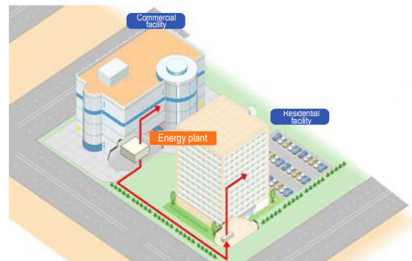
Figure 11 Point heating/cooling systems
