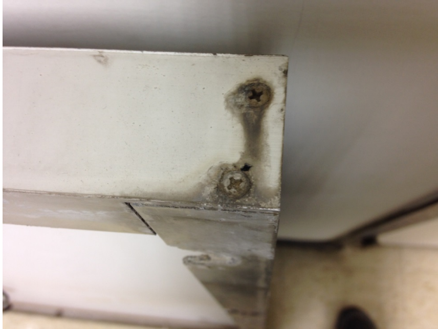
Figure 2.1.5.1.1 Aging module is assembled by screw
