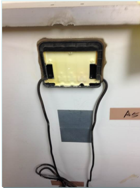
Figure 2.1.7.1 Diode and polymeric materials status inside the box
