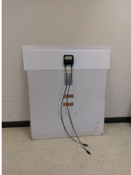
Figure 3.1.1.1 Laminate new EVA and Backsheet and install new junction box
