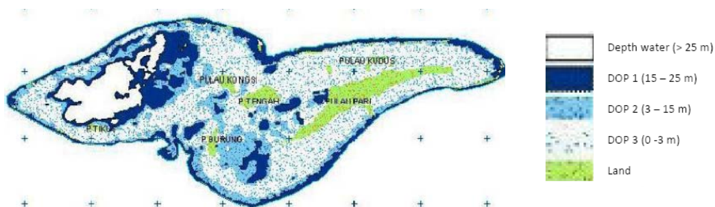
Figure 10: Result of depth chart using DOP of Jupp (1988) has resulted 4 depth classes.
