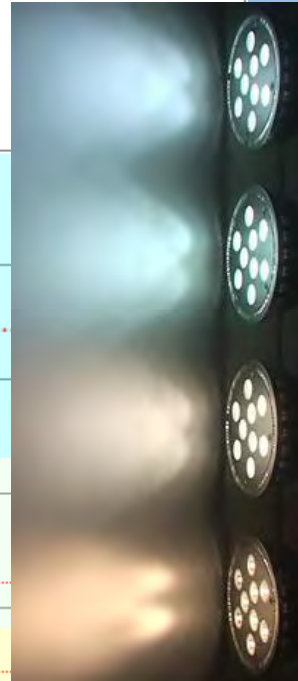
LED Correlated Colour Temperature (CCT) - Rated Values and Test Values
