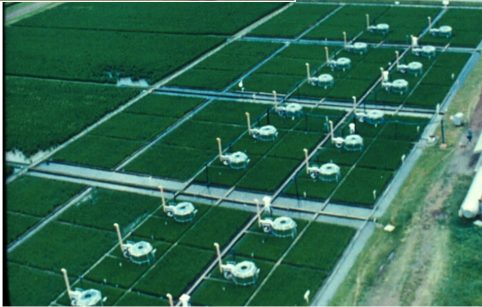
Open-top chambers (Temp./ CO2 effects)
